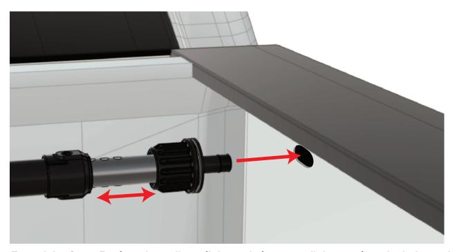
Extend the Cross Bar into the walls until the end pins pass all the way into the holes on both sides. The rubber pads will be flush to both walls.
