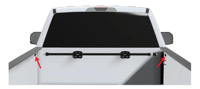
Cross Bar end pins will install through the bed wall. Locate the holes on the bed wall near the cab as shown above. Most trucks have them. If yours does not, You can make your own 11/16" holes or contact RIDE88 for other mounting hardware options.
