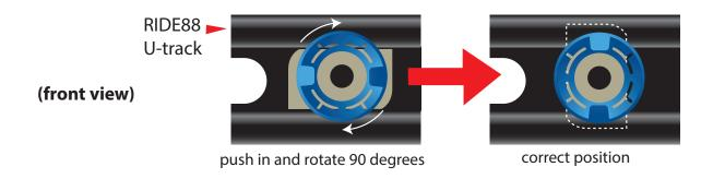
Install Single Mounts upside down as shown below if you have limited space due to some tonneau covers. This will allow clearance to open and close the cover when racks are folded down. If you do not have height restrictions, mount right side up.
