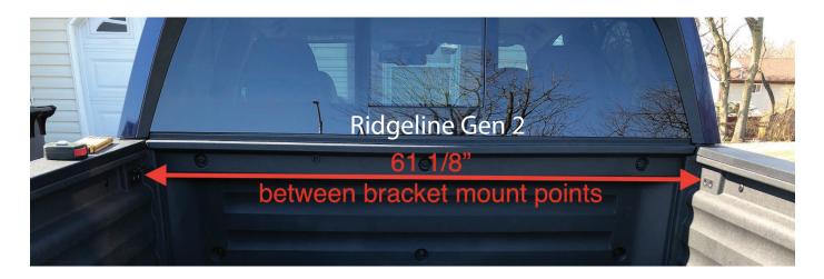
2. Confirm you have 90 degree bend Honda brackets installed
